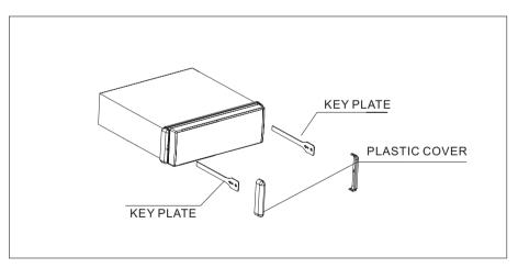
If you want to take CHASSIS out of the SLIDE BRACKET HOUSING, first remove the PLASTIC COVER of the both sides away, then insert the two KEY PLATE into left and right side of chassis as above illustration.
